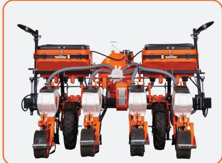
Increased gearbox height with close-type cover design prevents dust entry, ensuring smoother operation and longer gearbox life.
