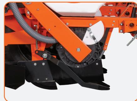
Lower seeder unit height keeps the seed drop point closer to the soil, so seeds enter the furrow with less bounce and roll, resulting in more accurate placement and uniform emergence.
