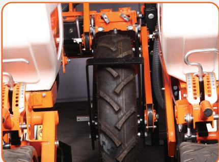
The rear fixed / floating type wheel to ensure proper ground contact during the cross bund and uneven field to avoid the seed missing and improve the seed accuracy.
