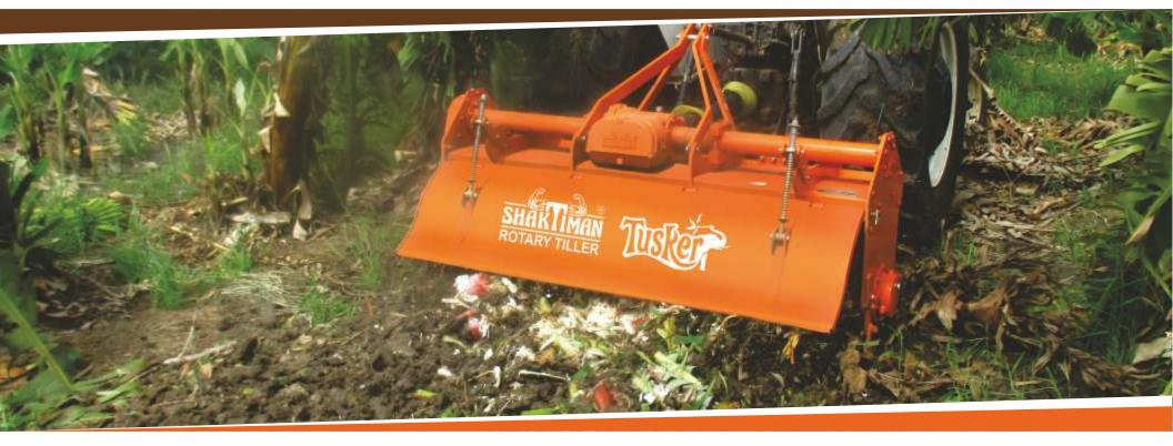
Tusker Series Rotary Tiller is specially designed for crushing of banana stem and pulverizes it within soil in a single pass. It is suitable for slashing thick and fibrous residue of crops such as banana, papaya, sugarcane etc. Pulverization of the crop
