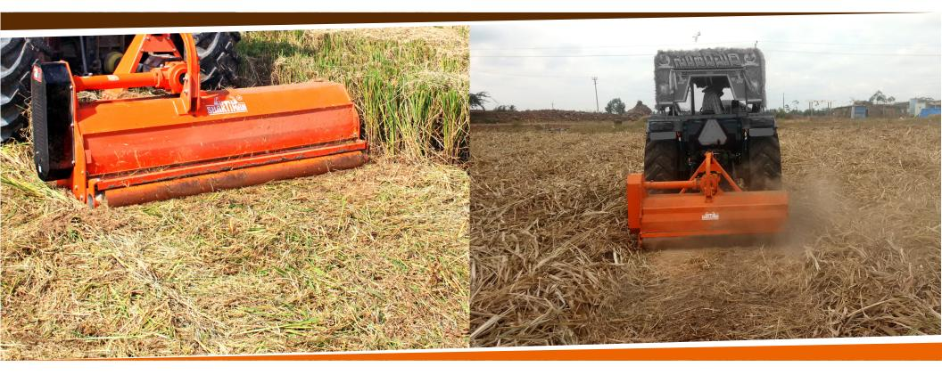
**SHAKTIMAN** Rotary Mulcher is robust & reliable implement to get rid off from crop residues like paddy straw, sugarcane trash, Maize stem etc. It is one of the best machine of its kind. It cuts and shred farm residues in small pieces and spread them in the field. The shredded particles work as a bio-mulch specifically for ratoon sugarcane and zero tillage sowing. It
