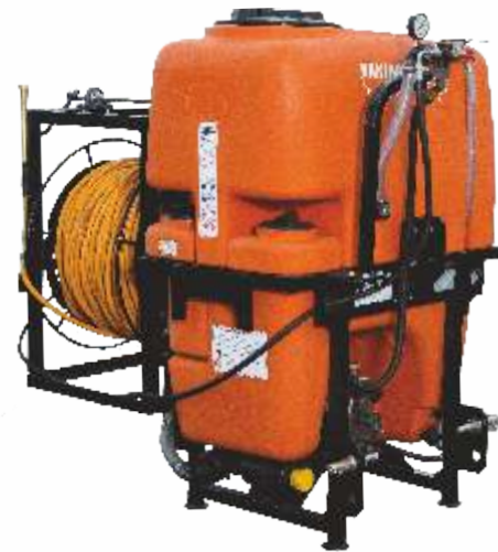
RAKSHAK with back Hose Reel & Spray Gun
