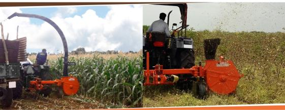
SHAKTIMAN Mobile Shredder is a tractor operated agricultural equipment for cutting and shredding crop stalks to clear the field faster for next crop. Suitable for row crops like cotton, castor, maize, chilli and other similar crops. Machine can be operated by any 40 and above hp tractor with dual clutch, attached to 3 point linkage and powered by PTO with \$40/1,000 rpm through driveshaft.
