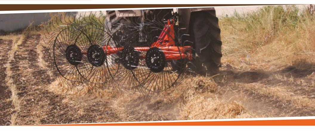
**SHAKTIMAN** Hay Rake is designed to move the mowed windrow across the soil surface or remaining crop stubble, creating a narrower windrow that will dry more rapidly.
